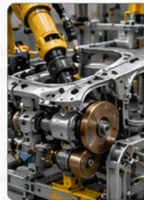
6 HEMMING & FLANGING Servo-driven rollers shape flanges and hems with closed-loop pressure and position control.
