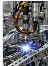
4 MIG WELDING & SEALING Multi-axis robots perform MIG welding and apply sealant with laser seam tracking.
