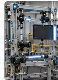
8 QUALITY INSPECTION Machine vision checks weld quality, gaps, flushness and hole presence.
