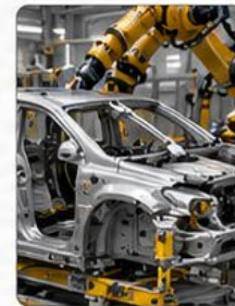
7 ROOF & SIDE ASSEMBLY Robotic handling and servo clamps assemble large sub-assemblies with high accuracy.
