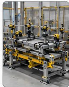
1 BODY LOAD IN Hydraulic lifts and precision locating pins position the body-in-white on the transfer fixture.
