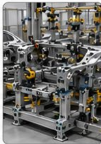
2 UNDERBODY FIXTURE Servo clamps and adjustable supports ensure repeatable and accurate body positioning.
